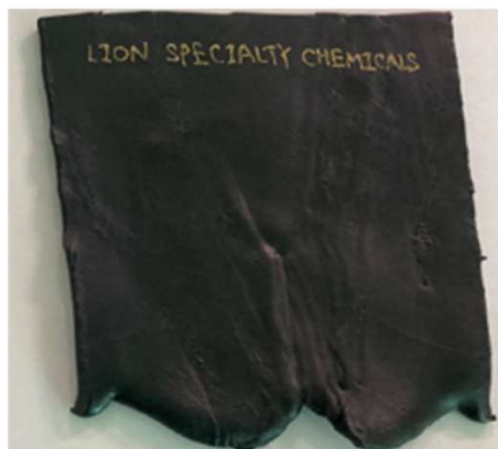
Rubber after being Dipped in GY-3660 (8%)
